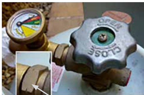
The nicks in the nut denote left hand thread
